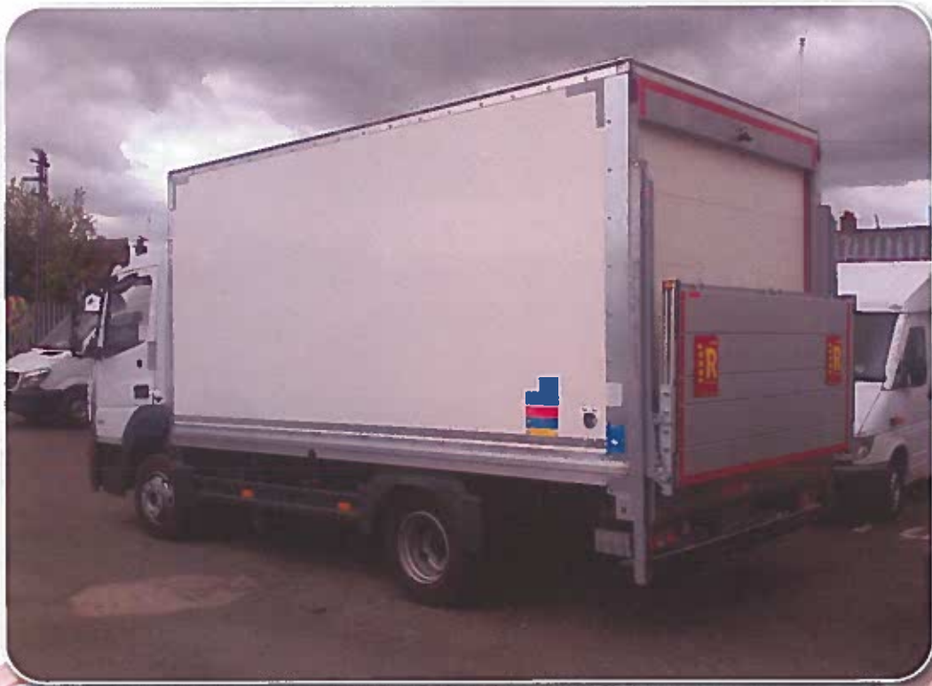
7.5 ton box body with tail lift and security enhancements
