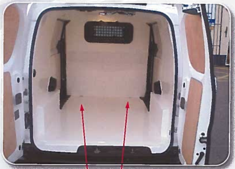
GRP lined with drains
